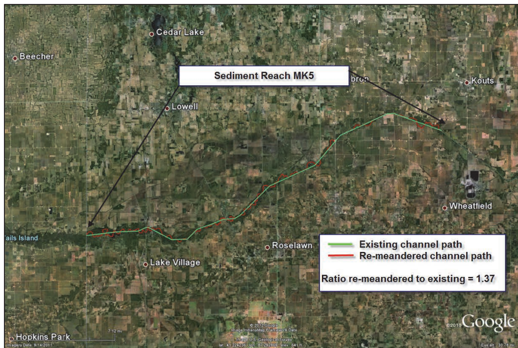
Figure 5.1. Assumed channel re-meander path for sediment reach MK5.
